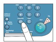
If Department ID Management is set, it is necessary to enter an ID and password. (If an optional Card Reader-E1 is attached, insert a control card.)
